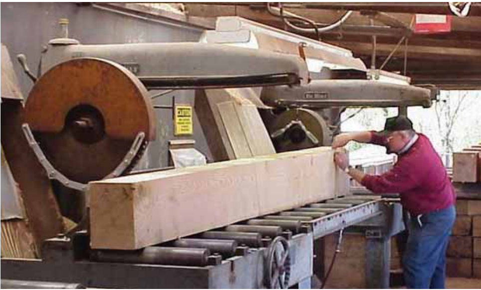
Measuring Timber for Dapping Photo by Phil Corder
