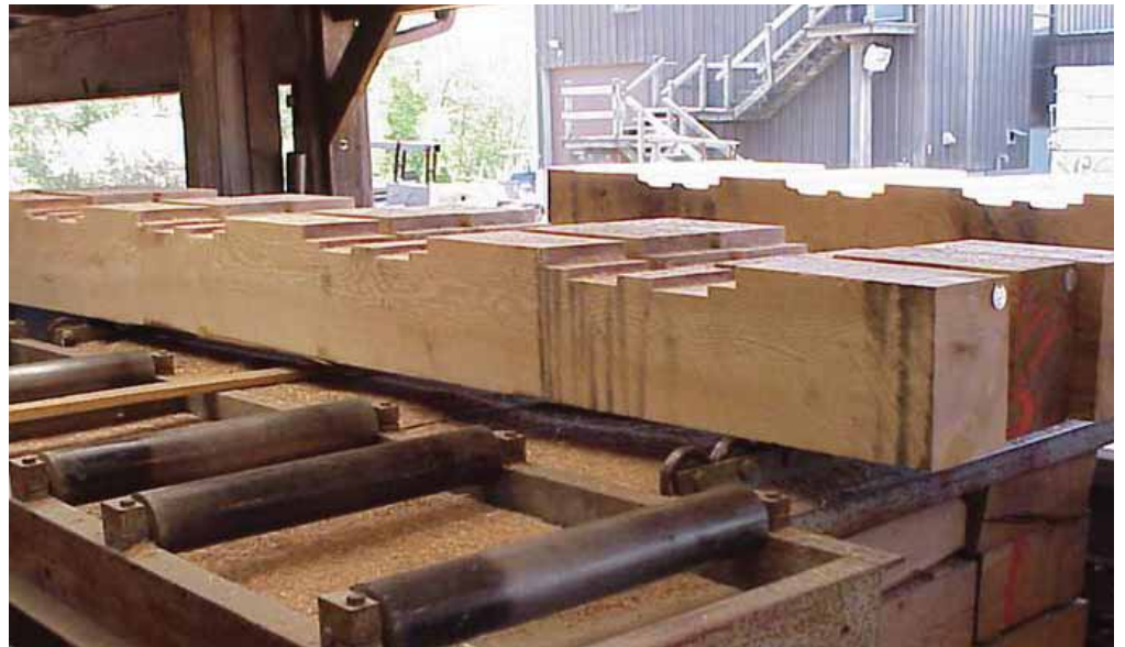
Dapped Bridge Timbers Photo by Phil Corder
