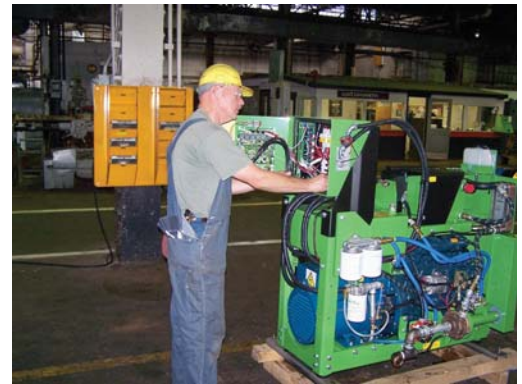
Electrician David Dyer prepares an APU for installation into locomotive 345. Photo by Mike Slaney
