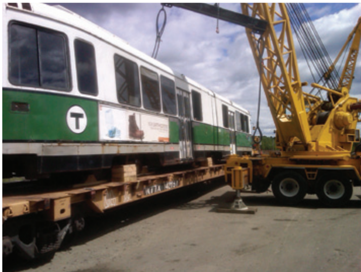
Pan Am's RC-130 mobile crane unhooking after lift of MBTA Green Line articulated trolley.
