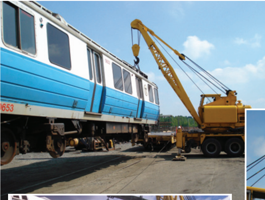
Winching TTX flat car underneath hoisted Blue Line Trolley
